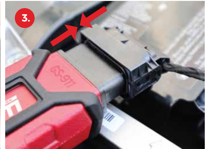
Insert the GS-911 male connector into the motorcycle's OBD-II female diagnostic port.
